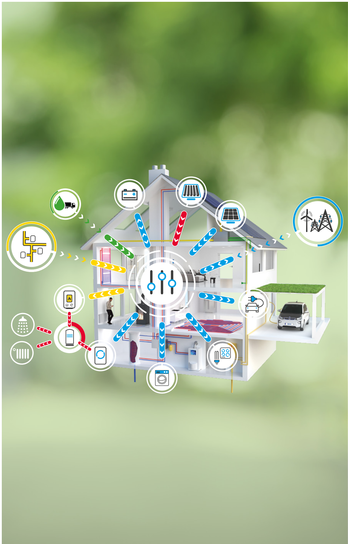
Networking of energy-relevant products with an intelligent energy management system (EMS)
