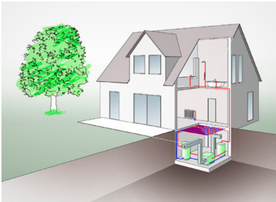
Air-water heat pump/monobloc installed indoors
